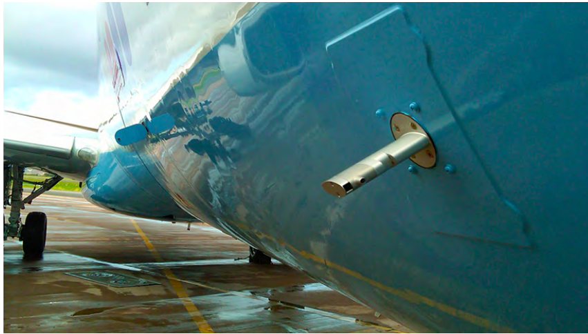
Figure 9: A TAMDAR sensor installed on the airframe of a jet aircraft (Panasonic, 2016).
