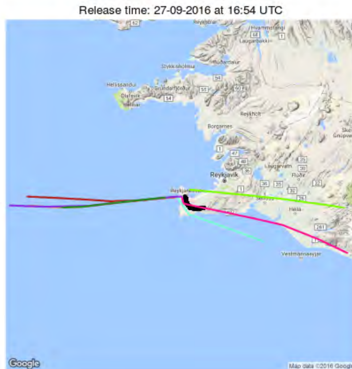
Figure 12: The tracks of TAMDAR flights (coloured) registered within the airspace shown and in the time frame of the radiosonde launched at 16:54 UTC on 27 September 2016, along with the trajectory of the radiosonde (black).
