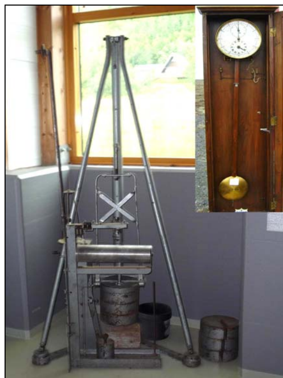
Figure 1: Photograph of a Mainka 135 kg horizontal pendulum, the second seismograph in Iceland and now on display at the Skógar Museum in southern Iceland. The inset photograph shows the contact clock from ISA, now at Icelandic Meteorological Office, which was used to time the measurements.
